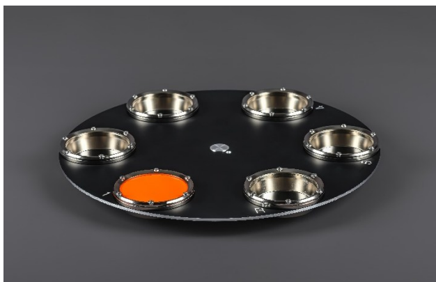
Fig. 1: Permeability dishes with a fixture to hold the film tightly sealed on top.
