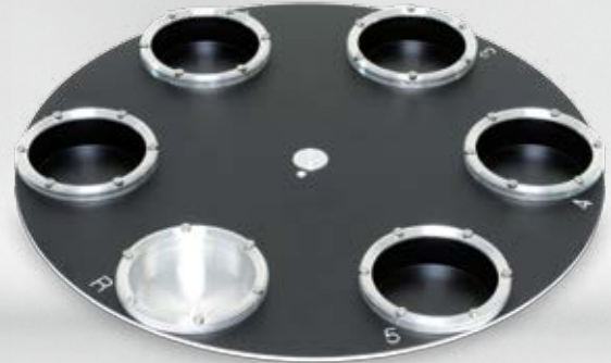
Permeability Kit, 5 samples Ø 80 mm, 1 reference Permeabilitätskit, 5 Proben Ø 80 mm, 1 Referenz
