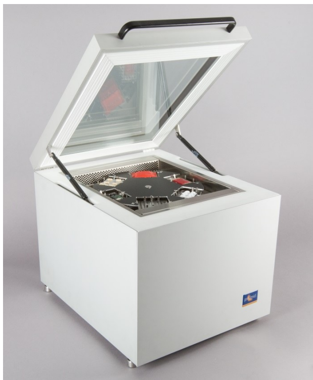
Fig. 1: SPS with Large Object tray with 5 sample positions and one reference pan for moisture sorption analysis of product packages.
