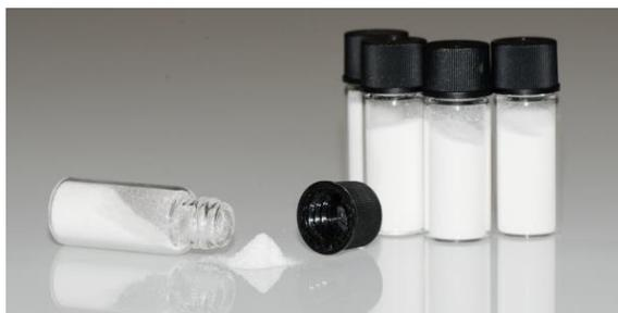
Fig. 1: Microcrystalline cellulose bottled in 2 ml vials for certification.
