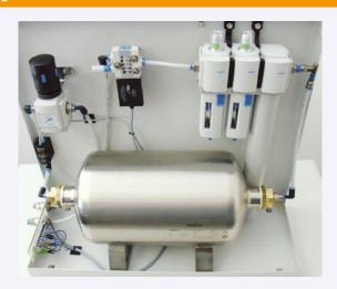
The Membrane dryer is installed between the SPS/Vsorp instrument and the local compressed air network in case the requirements for sufficiently dry air are not fulfilled. The entering air is filtered, dried and stored in a pressure tank. The membrane dryer meets the requirements of the SPS/Vsorp instruments for a pulse-proof compressed air supply.
