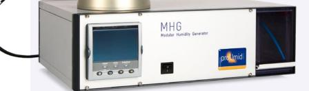
Moisture equilibration of powders, granules or pellets at controlled relative humidity. The powder conditioner is connected
