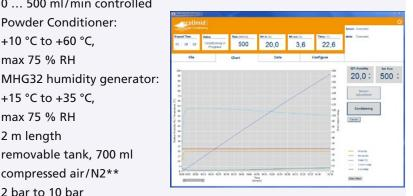
2 bar to 10 bar dry, clean, oil-free (class 1, ISO 8573-1:2010) MHG32: 100-120 VAC and 200-240 VAC, 50-60 Hz, 180 W Powder Conditioner: USB interface for the operation of the Powder Conditioner with the ProUmid MHG32 humidity generator. Computer is not included. operating system Windows 7/Windows 10
